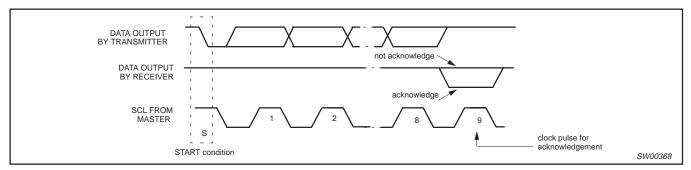
Figure 9. Acknowledgement on the I<sup>2</sup>C-bus
