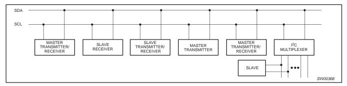
Figure 8. System configuration
