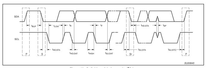
Figure 13. Definition of timing on the I<sup>2</sup>C-bus
