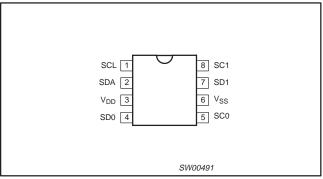
Figure 1. Pin configuration
