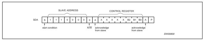
Figure 10. WRITE control register
